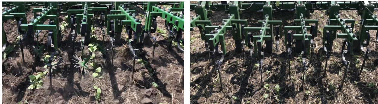
Figure 1: Camera-guided inter-row cultivator configured for wide rows with finger weeders (left), and configured for narrow 6" rows (right). Carman Manitoba, 2019.
